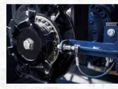
Consistently high throughput thanks to effective shredding in both directions of rotation, even when one shaft stops.
